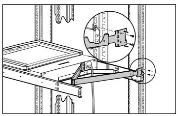
Figure 2-9. Attaching the cable management arm to the rear of the rack
